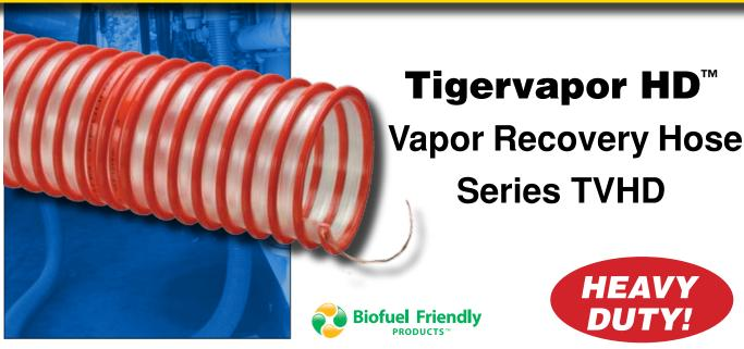
General Applications: Tank truck and terminal vapor recovery transfer Construction: Polyurethane hose with rigid PVC helix Service Temperature: -40°F (-40°C) to 150°F (+65.5°C)\*
