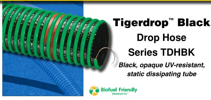
General Applications: Tank truck gravity drop fuel transfer Construction: Polyurethane hose with polyester fabric reinforcement and rigid PVC helix Service Temperature: -40°F (-40°C) to 150°F (+65.5°C)\*
