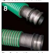
Step 8 — Insert the coupler's barbed shank into the hose, twisting counterclockwise as it enters. For ease of installation, an appropriate lubricant may
