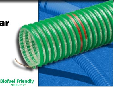
General Applications: Tank truck gravity drop and terminal fuel transfer Construction: Polyurethane hose with polyester fabric reinforcement and rigid PVC helix Service Temperature: -40°F (-40°C) to 150°F (+65.5°C)\*
