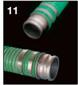
Step 11 — Install two hose clamps over the hose end above the coupling. The clamp buckles should be located 180° apart. When using banding coils, be sure to tighten clamps in a clockwise direction so the banding coils tighten down on the
