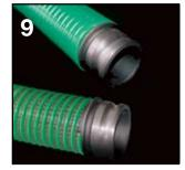
Step 9 — Insert the coupler into the hose until the hose seats against the bottom of the coupler.
