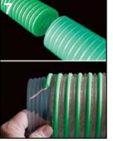
Step 7 — Screw approximately 12" of banding sleeve onto the hose; use appropriate lubricant as needed. Or, thread the banding coil between the helixes onto the hose. Slip the banding clamps onto the hose. TIP: When using banding coils, tighten clamps in a clockwise direction so the banding coil tightens down on the hose.
