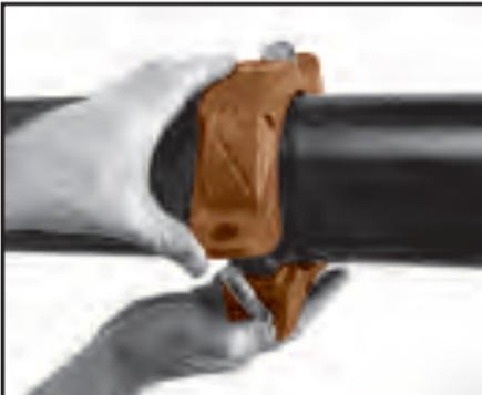
**4 Housings—** Remove one nut and bolt and loosen the other nut. Place one housing over the gasket, making sure the housing keys fit into the tube grooves. Swing the other housing over the gasket and into the grooves on both tubes, making sure the tongue and recess of each housing is properly mated. Re-insert the bolt and run-up both nuts finger tight.
