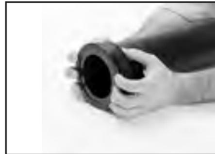
**1** Make certain the pipe ends are free of indentations, projections or other imperfections, which could prevent proper sealing of the gasket. Mark each pipe at a distance from the end of the pipe according to the pipe size:
