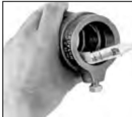
**1** Pipe surface shall be cleaned at least 1" from the end of the pipe to remove any coating, indentations, projections, and sharp edges which could affect proper gasket sealing. As a guide for installation, mark the pipe at a distance of 1½" from the end for 1", 1¼", and 1½" size fittings and 1¾" for the 2" & 2½" size fittings.
