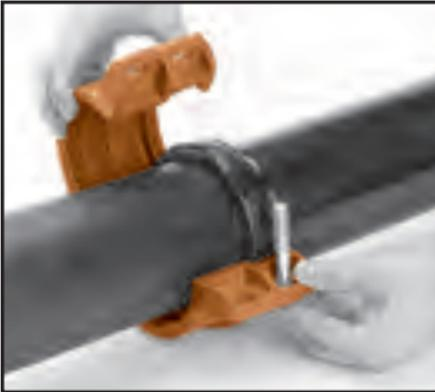
**4** Place each half of the coupling housing over the gasket, making sure the housing grooved end is directed into the pipe groove.
