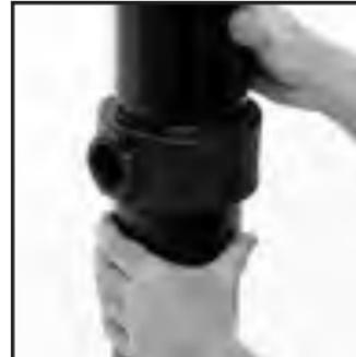
**3 Alignment**—Align the pipe ends and pull the pipe into the gasket until the center ribs are in contact with the pipe ends. The gasket should not extend into the groove on either pipe. Rotate the gasket to align the outlet of the gasket to the same direction as the branch outlet.
