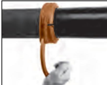
**5 Lock coupling**—Fit the nose of the locking handle in the notch of the opposite housing. Press firmly down on the handle until it makes contact with the coupling housing. Insert locking pin into handle linkage to secure handle in closed position. (See Caution.)
