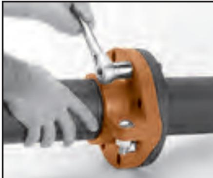
**5** Position the Gruvlok Flange gasket around the pipe end and press the gasket into the flange gasket pocket. Be sure the flange sealing lips are facing out.
