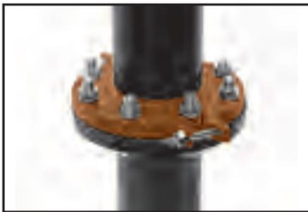
**7** Insert a flange bolt or stud with material properties of SAE J429 Grade 5 or higher through the bolt holes and thread a nut on hand tight. Continue this procedure until all bolt holes have been fitted. Tighten the nuts alternately and evenly so the flange faces remain parallel. All the bolts or studs must be torqued to the mating flange bolts specified torque. The flange faces should have metal-to-metal contact.
