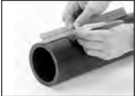
**1** Make certain the HDPE pipe end is square cut to  $\frac{1}{8}$ " maximum for the 2" to 4" and  $\frac{5}{32}$ " maximum for the 6" and larger sizes. The steel pipe must be grooved in accordance with Gruvlok® Grooving Specifications for Steel Pipe. The pipe ends must be free of scratches, indentations, projections or other imperfections, which could prevent proper sealing of the gasket.
