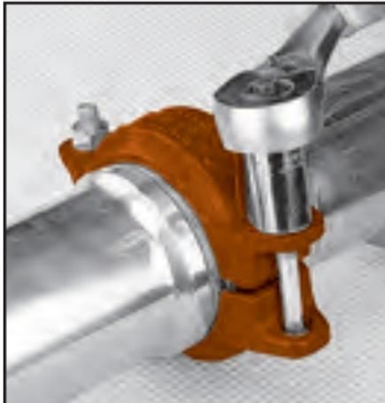
**4 Housings—** Remove one nut and bolt and loosen the other nut. Place one housing over the gasket, making sure the housing keys fit into the tube grooves. Swing the other housing over the gasket and into the grooves on both tubes, making sure the tongue and recess of each housing is properly mated. Re-insert the bolt and run-up both nuts finger tight.
