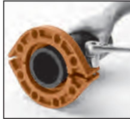
**4** Tighten the housing nut until the housing bolt pads make firm metal to metal contact. Torque all bolts to the required latch bolt torque levels. Refer to the Specified Latch Bolt Torque Table.
