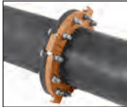
**5** Tighten the nuts evenly to the specified mating face bolt torque so that the flange faces remain parallel and make firm even contact around the entire flange.
