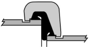
The centering rib allows for pipe positioning and serves to keep the smaller pipe from telescoping during installation. Used only with the Fig. 7010 Reducing Coupling.
