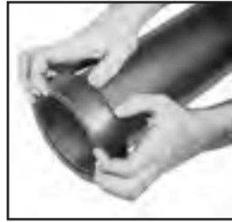
**3** Check the gasket color code to verify that the gasket grade is properly suited for the intended service. Apply a thin coating of Gruvlok Lubricant to the gasket lips and outside of the gasket and slip the gasket over one pipe. Make sure the gasket does not overhang the pipe end.
