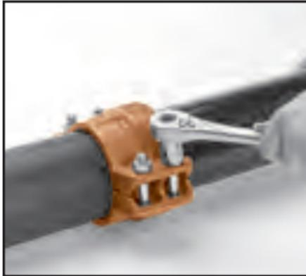
**5** Insert the bolts and secure the nuts alternately and uniformly until the bolt pads are in contact. Torque all bolts to the required bolt torque levels. Refer to the Specified Bolt Torque Table. There is no gap between the bolt pads and the bolt torque should be within the range given when the coupling is properly assembled. Alternate and even tightening of the bolts will significantly reduce the torque needed to close the gap at the pipe joint.
