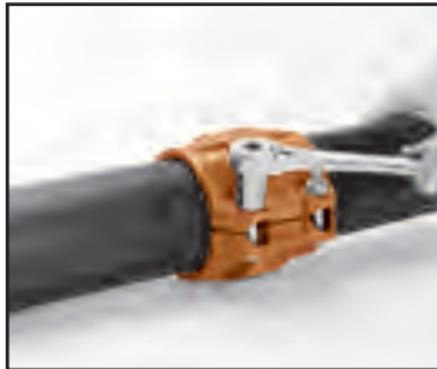
**5** Insert the bolts and secure the nuts alternately and uniformly until the bolt pads are in contact. Torque all bolts to the required bolt torque levels. Refer to the Specified Bolt Torque Table. There is no gap between the bolt pads and the bolt torque should be within the range given when the coupling is properly assembled. Alternate and even tightening of the bolts will significantly reduce the torque needed to close the gap at the pipe joint.
