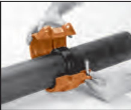
**4** Place the Figure 7305 housing casting over the gasket, making sure the tongue on one casting is aligned with the recess of the other casting.
