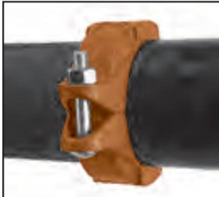
**4 Housings—** Place the coupling housing halves over the gasket making sure the housing keys engage the grooves. Insert bolts and turn nuts finger tight.
