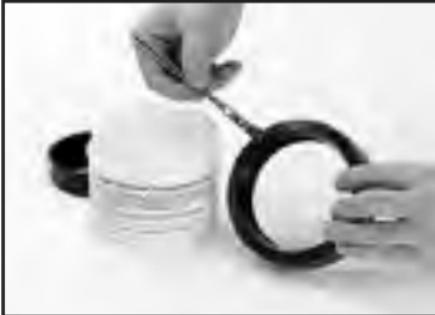
**2** Check to assure the gasket material is acceptable for the intended service. The Gasket color code is green for EPDM and orange for Nitrile (Buna-N).
