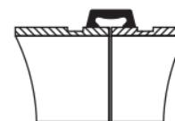
**NOTE:** The housings for sizes 16" and larger are cast in four or more segments.
