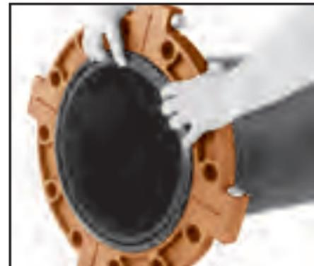
**1** Place each Gruvlok Flange segment around the grooved pipe with the key section fitting into the groove and the flange gasket cavity facing the pipe end. Loosely assemble the segments using the four segment-bolts-and-nuts. Alternately and equally tighten the latch bolts and nuts to the specified latch bolt torque bring the four flange segments into full, firm metal-to-metal contact.
