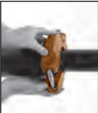
**4 Housings**—Place the coupling housing halves over the gasket making sure the housing keys engage the grooves. Insert bolts and turn nuts finger tight.
