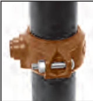
**5 Tighten Nuts**—Re-insert the bolt and run-up both nuts finger tight. Securely tighten the nuts alternately and equally until they are completely tightened and there is no gap between the bolt pads. Continue tightening the nuts alternately and equally until the specified bolt torque is reached.
