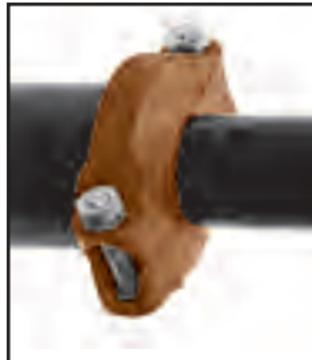
**6 Assembly Complete**—Visually inspect the pipe joint to assure the coupling keys are fully engaged in the pipe grooves and the bolt pads are in firm even metal-to-metal contact on both sides of the coupling.
