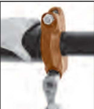
**5 Tighten Nuts**—Tighten the nuts alternately and equally to the specified bolt torque. The housing bolt pads must make metal-to-metal contact.
