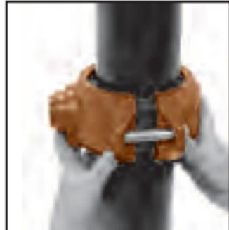
**4 Housing Assembly**—With one nut and bolt removed and the other loosened, place one side of the housing over the gasket. Make sure the ribs on the outside of the gasket align with the recesses in the housing and the keys in the housing are in the grooves on both pipes. Swing the other housing over the gasket and into the grooves on both sides of the pipe. Make sure the recess in the outlet of the housing is properly aligned with gasket outlet.
