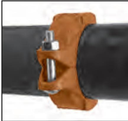
**4 Housings**— With one nut unthreaded to the end of the bolt, unthread the other nut completely and swing the coupling housing halves over the gasket, making sure the housing keys engage the grooves. Insert the bolt and turn the nuts finger tight.
