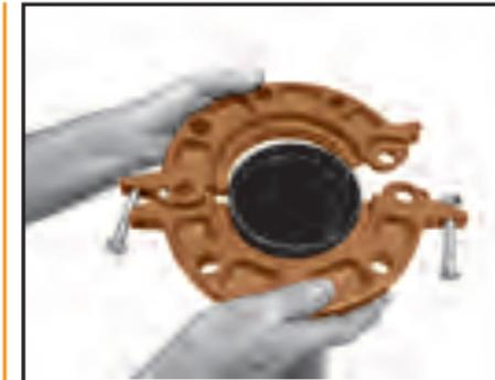
1 On the side without the hinge pin, loosen the latch bolt nut to the end of the bolt thread. (It is not necessary to remove the nut from the latch bolt.) Swing the latch bolt out of the slot. Open the Gruvlok Flange and place around the grooved pipe end with the key section fitting into the groove. The flange gasket cavity must face the pipe end.
