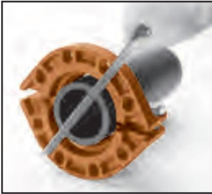
**3** Place the housing over the end of the pipe and using a straight edge, align the face and the flange face with the end of the pipe. Do not let the pipe extend beyond the flange face.
