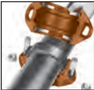
**5** Place each half of the Roughneck coupling over the gasket, making sure that the tongue on one housing half is aligned with the recess on the other housing half.
