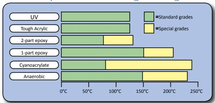
Products can withstand higher temperatures for brief periods providing joint is not unduly stressed.
