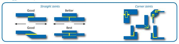
TIP: If joint design cannot be modified, opt to use a toughened adhesive with high peel strength.
